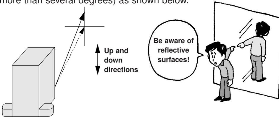
**2. Is the sensor detecting the surface on which it is installed?**
