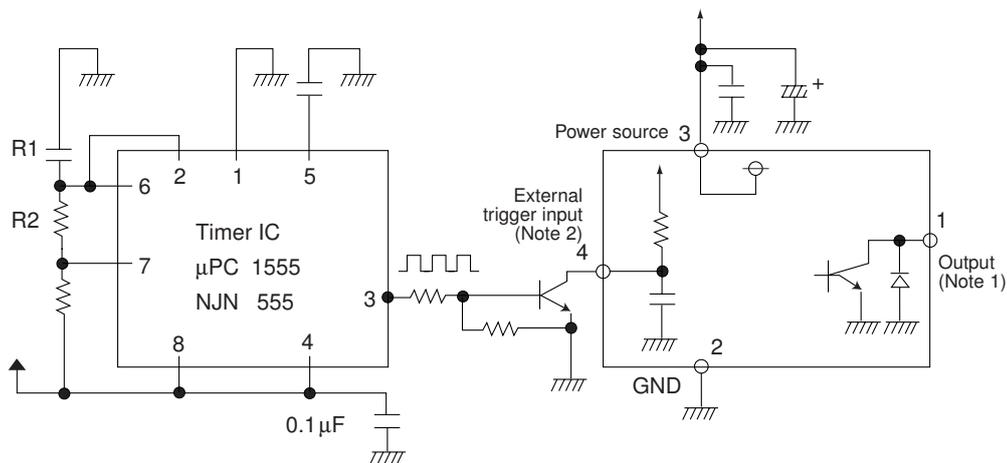
Notes: 1. The output transistor has an open collector structure.
