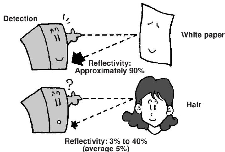
Why is a detection signal output even though no object is in the detection area?
