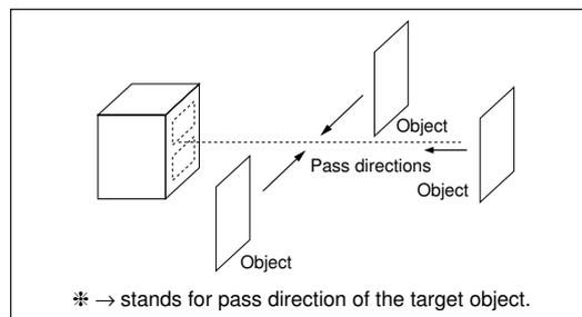
Install the sensor so that it points in the direction shown at left with respect to the direction of entry of the object.
