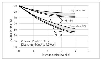
Self-discharge is affected by the temperature at which the batteries are left standing and the length of time during which they are left standing. It increases in proportion as the temperature or the shelf-standing time increases. Panasonic's Ni-MH batteries have excellent self-discharge characteristics.
