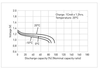
CHARGE METHODS FOR NI-MH BATTERIES 4
